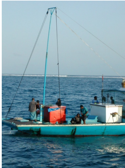
Figure 2: A fishing boat in Haa Alifu Atoll (North) with pulley system for large yellowfin tuna fishing (September 2004)
