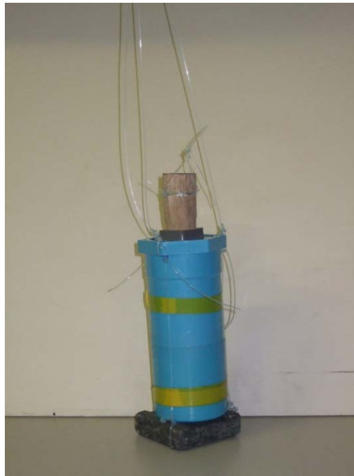
Photo 15. Modified Nansen bottle used for water collection in B. Kamadhoo
